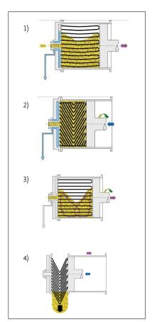
**Application** The HPS press was developed for the solid-liquid separation of biological substances. This machine is the effective solution for dewatering of communal and industrial sludge. The solid content of a suspension may be between 2 and 10%. For several performance requirements there are several machine sizes provided.
